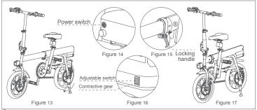
● Fold the kickstand, lower the head and saddle height to the minimum (see Figure 13). Turn on power (see Figure 14), release the locking handle (see Figure 15 - ® arrow); set right the body, put the adjustable switch in the contractive gear (see Figure 16). The body automatically folds, and when finishes, put the adjustable switch in the stop gear, close the locking handle, turn off the power (see Figure 17).
